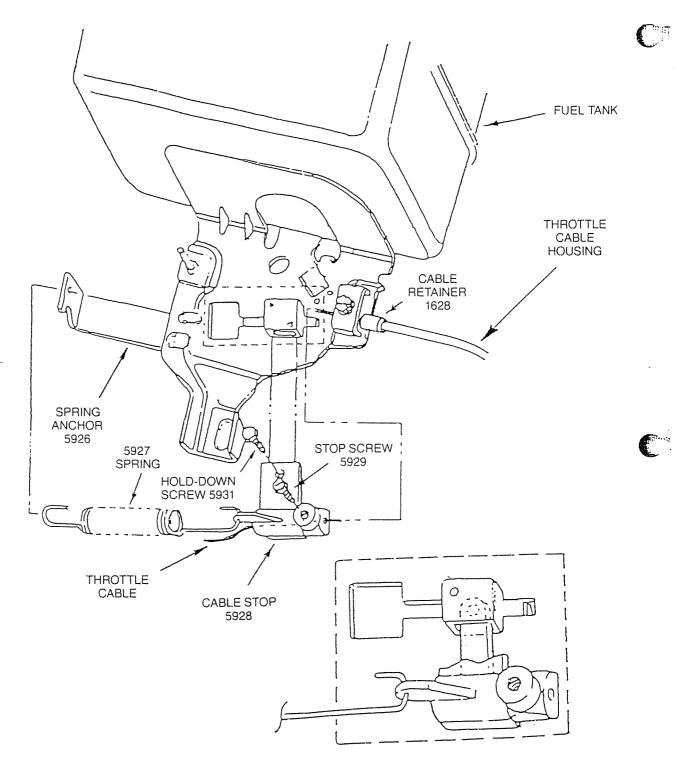
**ASSEMBLY:** Pass the throttle cable through the cable retainer and butt the throttle cable housing end against the inside shoulder of the cable retainer. (The cable retainer is to be securely fastened to the engine with the clamping screw.) Pass the end of the Throttle Cable through the hole in the cable stop. Before tightening cable stop screw:
