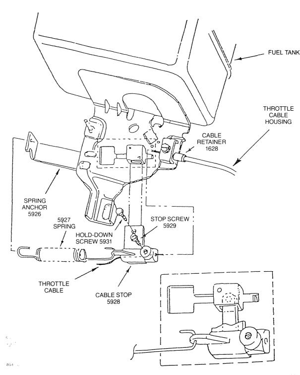
**ASSEMBLY:** Pass the throttle cable through the cable retainer and butt the throttle cable housing end against the inside shoulder of the cable retainer. (The cable retainer is to be securely fastened to the engine with the clamping screw.) Pass the end of the Throttle Cable through the hole in the cable stop. Before tightening cable stop screw:
