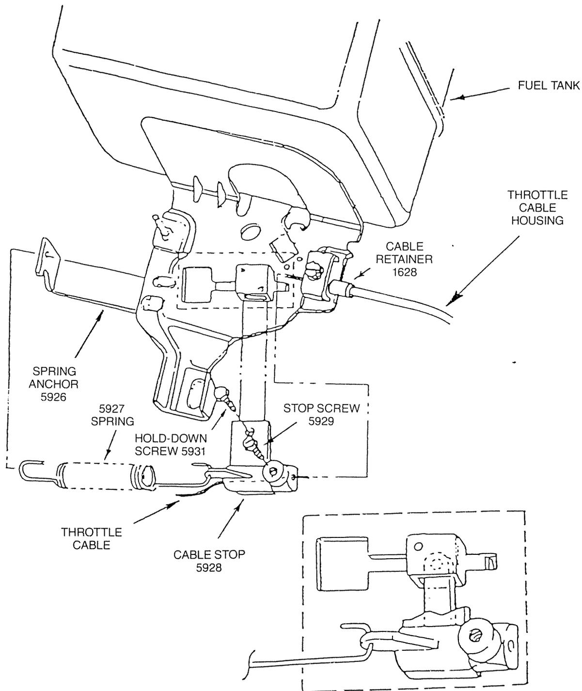
**ASSEMBLY:** Pass the throttle cable through the cable retainer and butt the throttle cable housing end against the inside shoulder of the cable retainer. (The cable retainer is to be securely fastened to the engine with the clamping screw.) Pass the end of the Throttle Cable through the hole in the cable stop. Before tightening cable stop screw:
