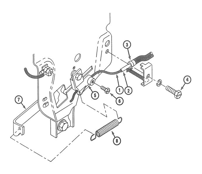
ASSEMBLY: Pass the Throttle Cable (Item 1) through the 1628 Cable Retainer (Item 2) and butt the Throttle Cable Housing End (Item 3) against the Inside Shoulder of the 1628 Cable Retainer (Item 2). The 1628 Cable Retainer (Item 2) is to be securely fastened to the engine with the Clamping Screw (Item 4). Pass the Wire End of the Throttle Cable Housing (Item 1) through the hole in the 5928 Cable Stop (Item 5). Before tightening 5929 Cable Stop Screw (Item 6):
