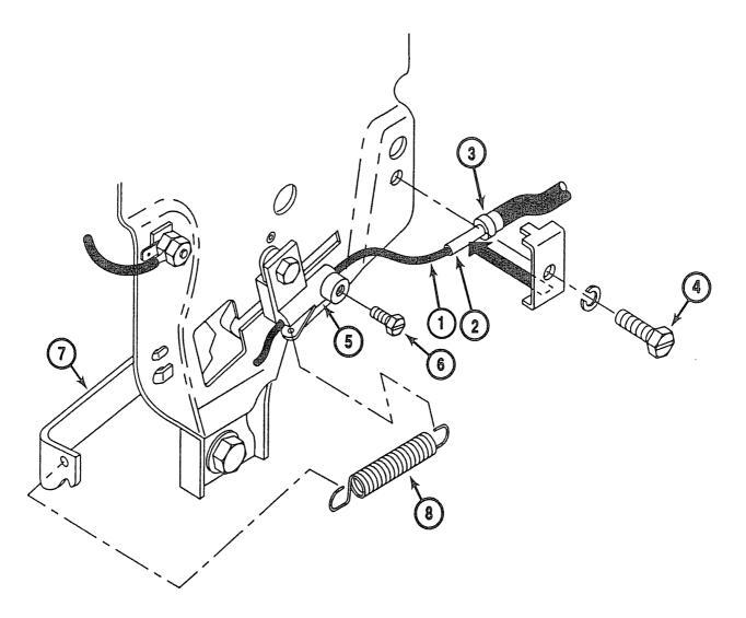
**ASSEMBLY:** Pass the Throttle Cable (Item 1) through the 1628 Cable Retainer (Item 2) and butt the Throttle Cable Housing End (Item 3) against the Inside Shoulder of the 1628 Cable Retainer (Item 2). The 1628 Cable Retainer (Item 2) is to be securely fastened to the engine with the Clamping Screw (Item 4). Pass the Wire End of the Throttle Cable Housing (Item 1) through the hole in the 5928 Cable Stop (Item 5). Before tightening 5929 Cable Stop Screw (Item 6):
