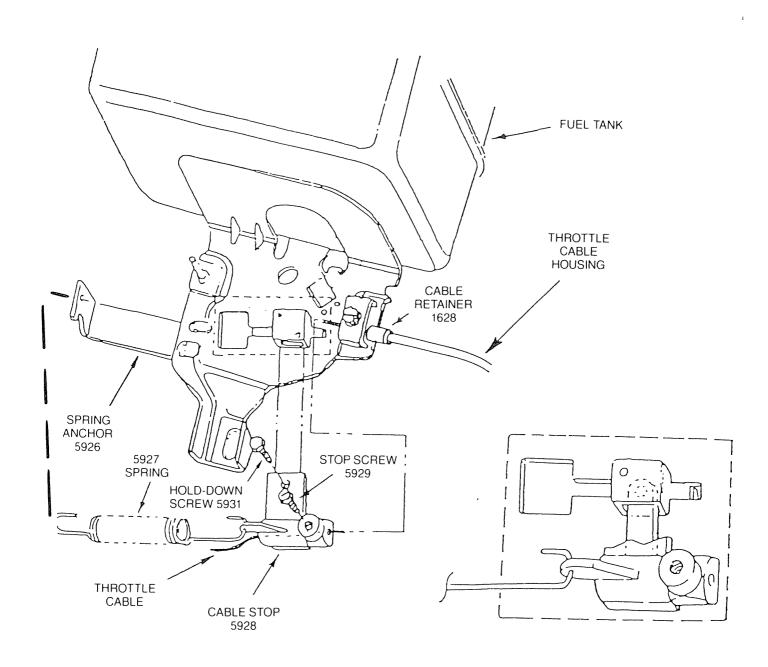
**ASSEMBLY:** Pass the throttle cable through the cable retainer and butt the throttle cable housing end against the inside shoulder of the cable retainer. (The cable retainer is to be securely fastened to the engine with the clamping screw.) Pass the end of the Throttle Cable through the hole in the cable stop. Before tightening cable stop screw:
