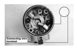
Inspect the conducting condition between the connecting wire terminal and the carbon brush. It should be conductive. Measure the length of the carbon brush. Replace it if it exceeds service limit.
