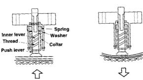
As for the adjustment of the cam chain tensioner, clockwise is tightening, and counterclockwise is loosening.
