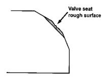
Ream the upper angles of the valve seat working surface with a 30° milling cutter.
