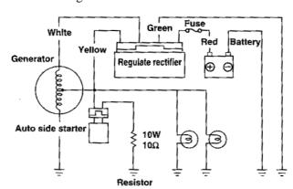
Measure the resistance value between the white wires of the generator and connecting wire of the vehicle body.
