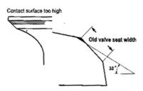
• Ream the lower angles of the valve seat working surface with a 60° milling cutter.
