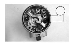
Inspect the needle bearing in the carbon brush base. It should be able to move smoothly with no play.
