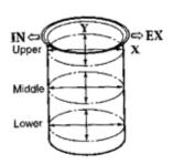
cross section, measured the difference of diameter between two points mutually perpendicular; which is the circularity of the cylinder.
