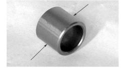
Inspect if there is any abrasion or damage of the drive plate hub.
