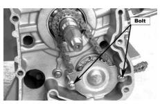
Remove the oil pump driving gear nuts, and remove the driving gear, chain.
