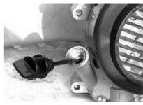
Allow time for oil to return to oil pan, then check oil level on the filler cap stick to assure proper level. The cap needs to be screwed in to check.
