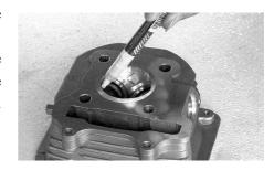
Before lapping, clean the valve, valve seat and valve guide.
