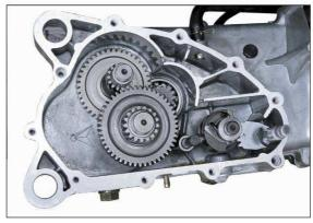
• Revolve the shift selector in proper to ensure that the mark on shift camshaft set in the middle of 2 marks on the shift selector exactly. That is the assembling of shift camshaft assy.
