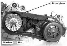
Do not allow any grease or oil on the surface of the movable drive plate and the driven belt.
