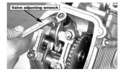
Sometimes, when tightening the locknuts the clearance will change, so it must be rechecked for the proper clearance.
