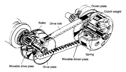
Its basic operational principle is to realize automatic CVT by the diameter changes (the transmission ratio changes) of the driving and driven belt pulley.
