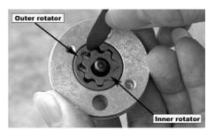
Inspect the clearance between the rotator plane and the oil pump.
