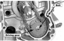
Remove the oil pump positioning bolts, and remove the oil pump assembly.
