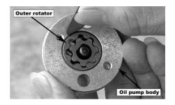
Inspect the clearance between the inner rotator and the outer rotator.
