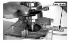
Mount new dowel pins and gasket on the left crankcase. Join the right crankcase and left crankcase together.
