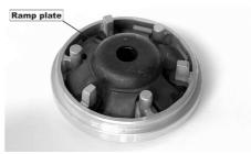
• Remove the centrifugal rollers.
