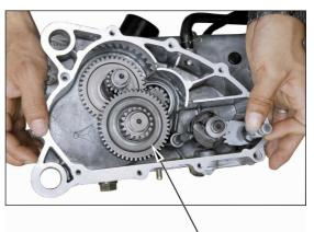
Gear Shifting Shaft Assembly
