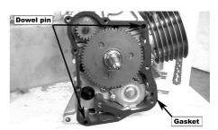
Remove the oil pump partition plate positioning bolts, and remove the oil pump partition plate.
