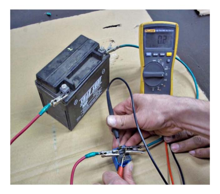
$\bullet$  Using the resistance setting on the multi-meter, check across posts 30 and 87.
