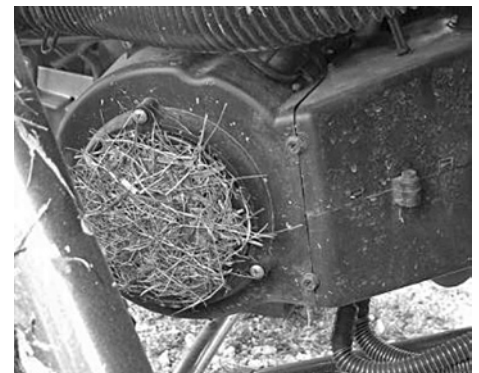
Debris clogging the cooling fan
