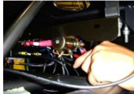
One (+) probe placement shown (either small post with an orange wire is acceptable)
